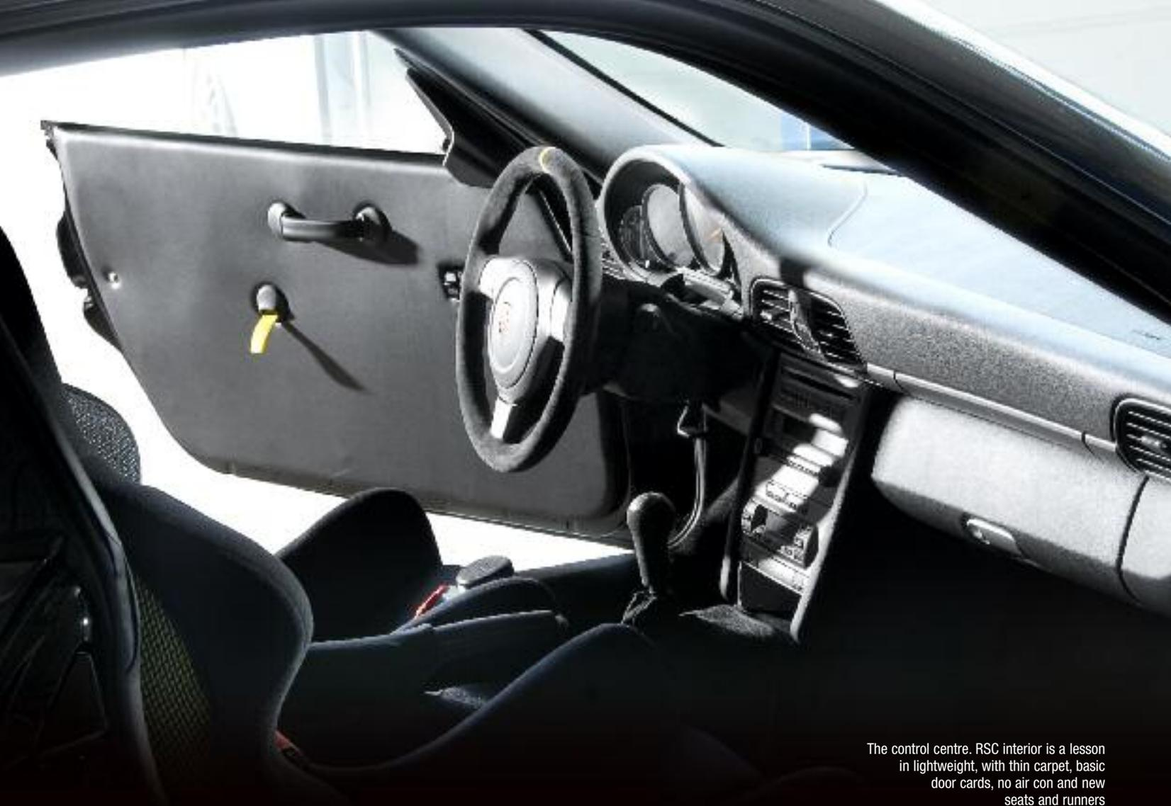
The control centre. RSC interior is a lesson in lightweight, with thin carpet, basic door cards, no air con and new seats and runners
