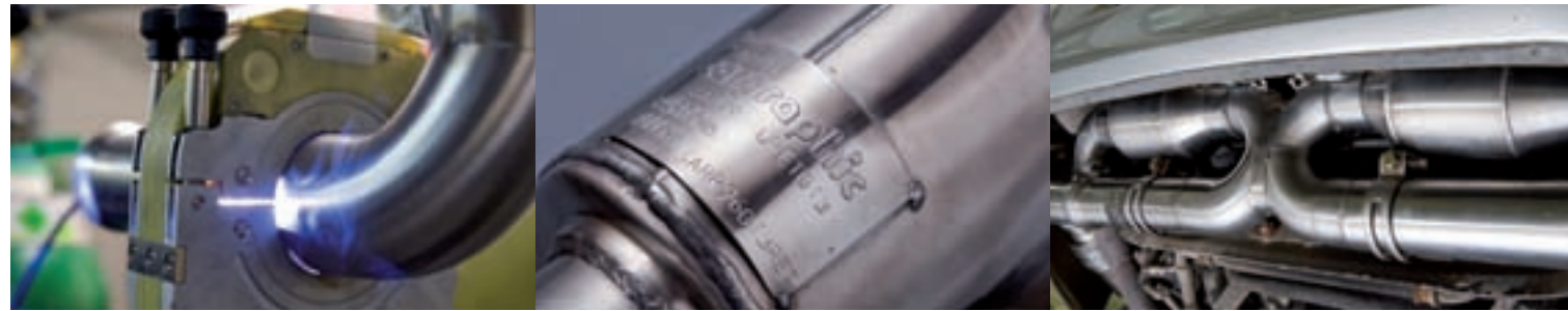
Above left to right: Tubes are argon filled during welding. All important ID plate, complete with TUV number. Jumping ahead somewhat, but exhaust in situ. It's a quality piece of kit. Below: Our exhaust fits the set-up jig like a glove
